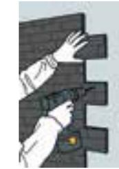
Place the panel on the wall and use the 3mm bit to drill through the joints across the panel till you get to mark the wall where wall plugs will be fixed later.
