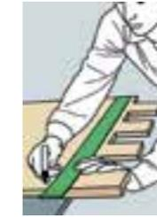
Use a ruler and a marker and draw a line along the surface to be cut.
