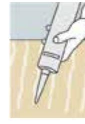
We will apply a few vertical lines of glue on the back of the panel. This is very important for panels installed outdoors
