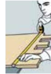
Measure the surface to be covered and calculate how many panels will be needed. Each one is approx. one square meter.
